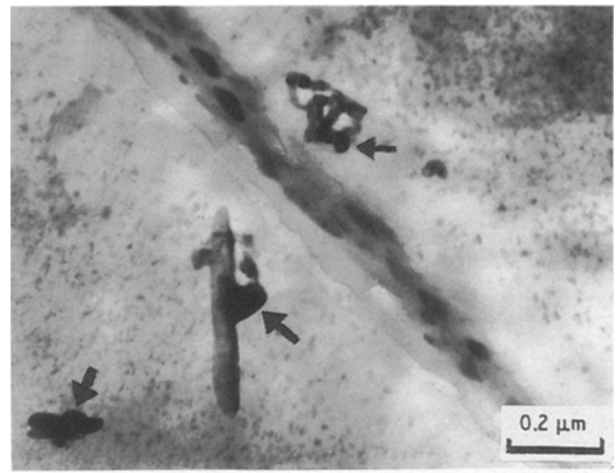
Figure 4 Tritium electron microautoradiograph of Al-6 wt % Zn-2 wt % Mg alloy aged at 160 °C for 10 ks after quenching. Silver grains are observed at the interface between the matrix and the unresolved rod-like \eta precipitates, as shown by arrows.
